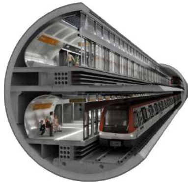
Barcelona Metro – Line 9 Tunnel with unique two-level design
